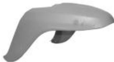
Body work, in reality the Lambretta is a brick in terms of weight and design of bodywork. Not only is the Lambretta not aerodynamic, but also heavy as well. Weight in terms of speed and acceleration also is a big deal in how well your scooter performs. There are many fibreglass, Kevlar and other such exotic panels appearing on the market that if you want to gain speed by saving weight, you can do so. The old joke that if you want to improve performance simply go on a diet is quite true!
