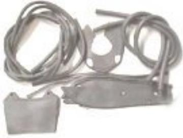
Rubber kit, which includes, front mudguard gaskets, horn cast side gaskets, horn cast base gasket, leg shield rubbers, side panel rubbers, rear light unit gasket (not in S1/2 kit), air scoop gasket, handle bar grips, and a brake pedal rubber.
