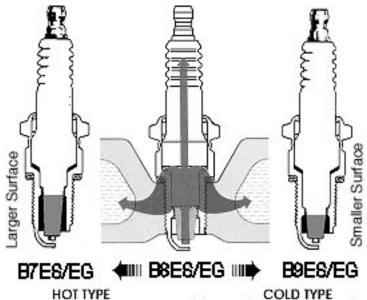
It has a larger surface exposed to the combustion gasses. It dissapates heat slowly. Its firing end heats up quickly
